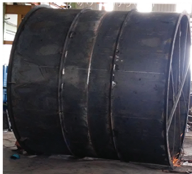
ENCASEMENT CONCRETE CASING
