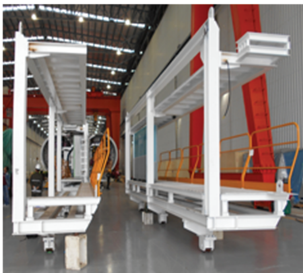
BACK-UP CAR FOR TBM
